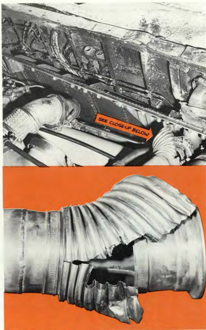
This is typical damage caused by a BLC duct failure (top). The actual failed duct is shown in the bottom photograph.
